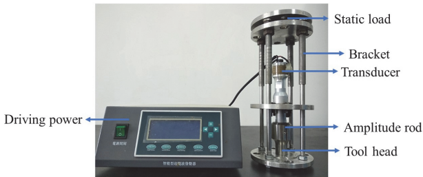
Figure 1 The piezoelectric ceramic ultrasonic vibration generator
