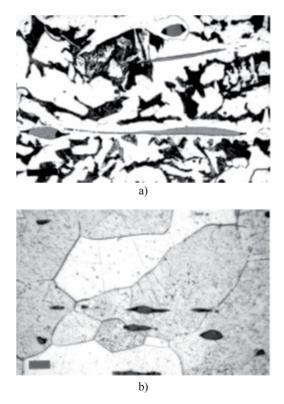
Fig. 3. The optical micrographs of: a) Brooklyn Bridge steel showing manganese sulfide (MnS), b) Springfield Barrel steel showing MnS inclusions with silicate ends [47]
