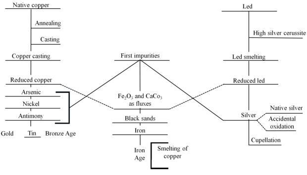
Fig. 1. Schematic tree of the development of metallurgy [11]
