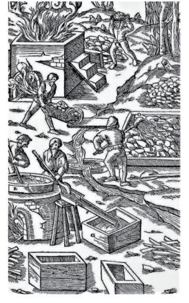
A – furnace, B – enclosed space, C – aluminous rock, D – deep ladle, E – caldron, F – launder, G - troughs
