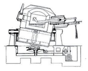
Fig. 4. Stassano furnace [48]
