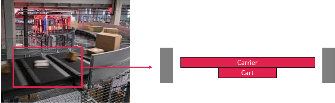
Figure 1.1: The sortation system (left) and a schematic representation of the cart and carrier (right)
