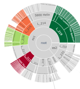
Figure 13: Visualisation for "Find the assets that are large consumers". This sunburst plot shows the assets with the highest consumption, using the radial angular spatial position. The colour is based on how much energy the loop consumes compared to the average. Red colours indicate over consumption, while green colours indicate under consumption.
