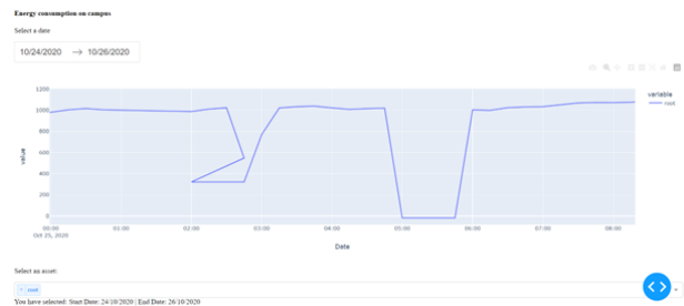
Figure 3: Night in 2020 in which the time was reverted from Daylight Saving Time to standard time. This figure shows that the data does not follow its usual pattern.
