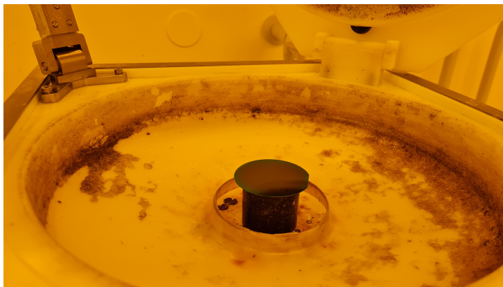
Figure A.4: Sample is located in the spinner to spin coat the resist, step 1c)
