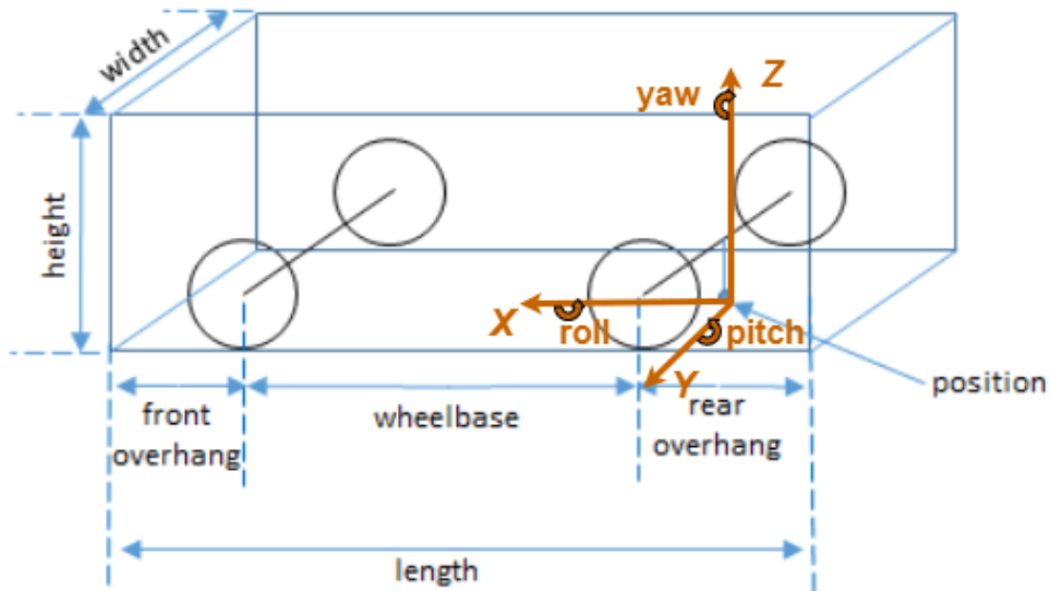
Figure 2.1: Ego vehicle and vehicle fixed coordinates (taken from mathworks.com )
