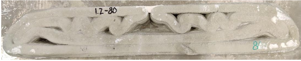
Figure 29 – Tested 630x100 beam (80%speed)
