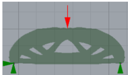
Figure 57 – Karamba optimised structure
