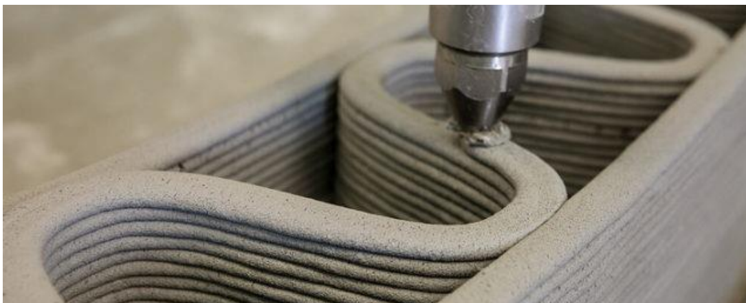
Figure 1 - 3d concrete printing
