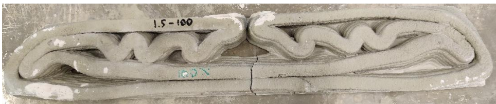
Figure 28 – Tested 630x100 beam (100%speed)
