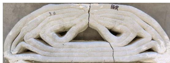
Figure 44- Unexpected failure (630x200v.2)
