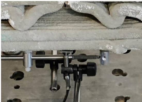
Figure 20 – LVDT placed on the structure
