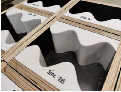
(a) Formwork used to cast specimen
