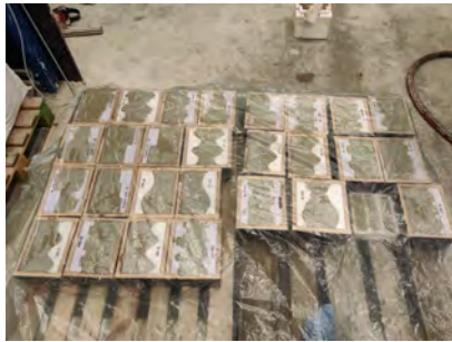
(c) Hardening while covered for first 24 hours
