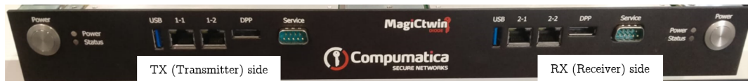
Figure 5.1: The front of the MagiCtwin Diode. On the left we have a power button and connection gates of the TX (transmitter) side. On the right we see the same for the RX (receiver) side.
