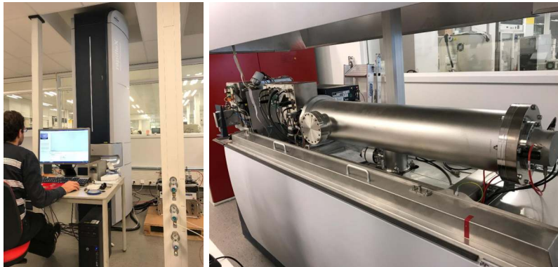
Figure 2.2 RapifleX time-of-flight MALDI-MSI equipment. The tower of ion detector/reflector with a 300-cm effective flight path (left photo). 3D laser-beam generator (right photo).
