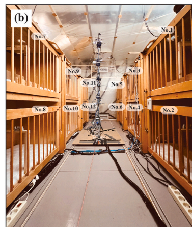
Fig. 1. Experimental setup. (a) Axonometric schematic of the full-scale bedroom, including 12 beds (from No.1 to No.12) and sensor placement. (b) A picture of the on-site bedroom.
