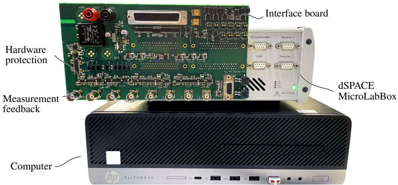
Figure 8.4 A photograph of the interface board with dSPACE MicroLabBox.
