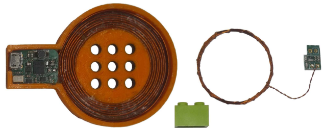
Fig. 6. Realized transmitter (left) and receiver (right) prototypes. Standard 2 \times 1 LEGO brick for size.
