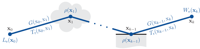
Figure 1: The measurement contribution function. A light path of k + 1 vertices and k segments is shown, with the first and last vertices being at the light source and the eye, respectively. The first scattering event occurs in a medium and the last on a surface.
