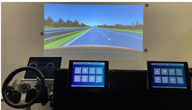
Figure 3. Demonstration of the simulator and study set-up with the mounted IVIS screens.
