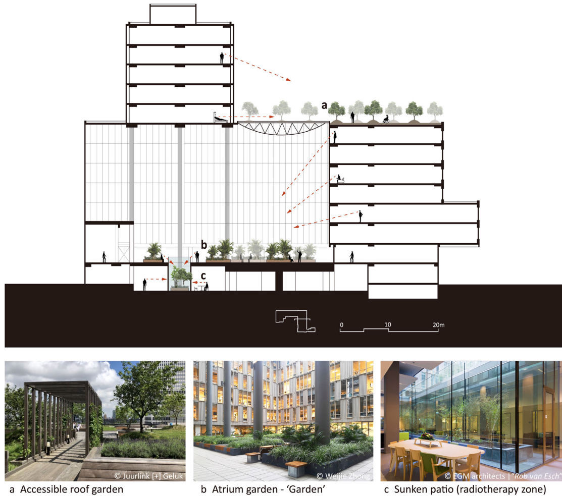
Fig. 7 Section and photographs of the three green pocket variations in Erasmus MC (section drawing source: authors, based on EGM architects and Juurlink [+] Geluk).
