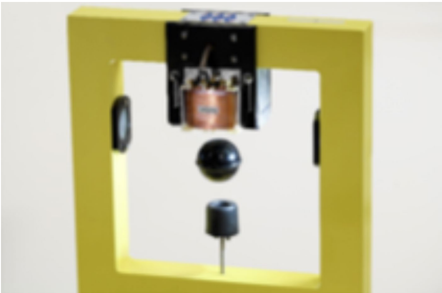
Fig. 2 Magnetic ball levitation set-up
