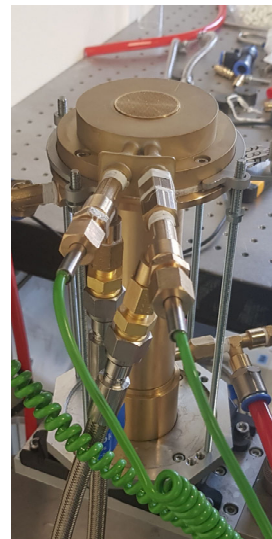
The adapted HFB. Installed with thermocouples, cooling and heating hoses.
