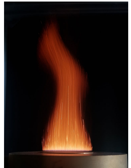
A hybrid methane-iron-air flame produced by the adapted HFB.
