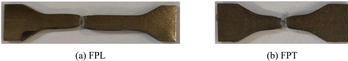
Figure 4-12. Fractured miniature flat plates for base metal.
