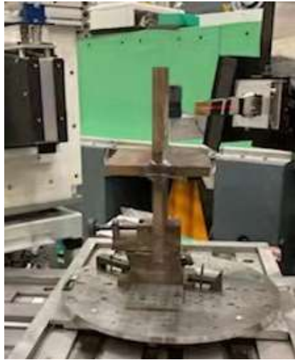
Figure 6-7. Photo of the test setup for longitudinal residual strain measurements of a fillet-welded specimen.
