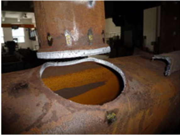
(a) Welded CHS-RHS joint [90]
