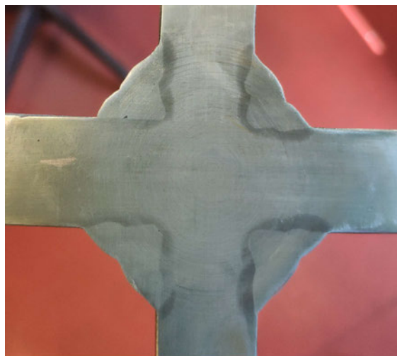
Figure 7-2. Photo of the macroetched surface of a F12 specimen.
