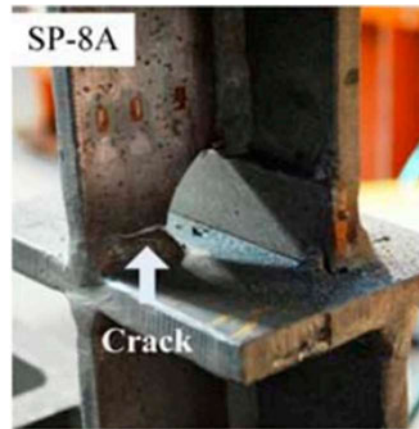
(b) Local welded connection [84]
