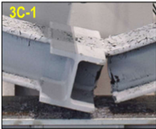
(e) H-section connections [94]
