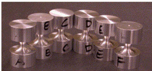
(e) Compression cylindrical specimens [27]
