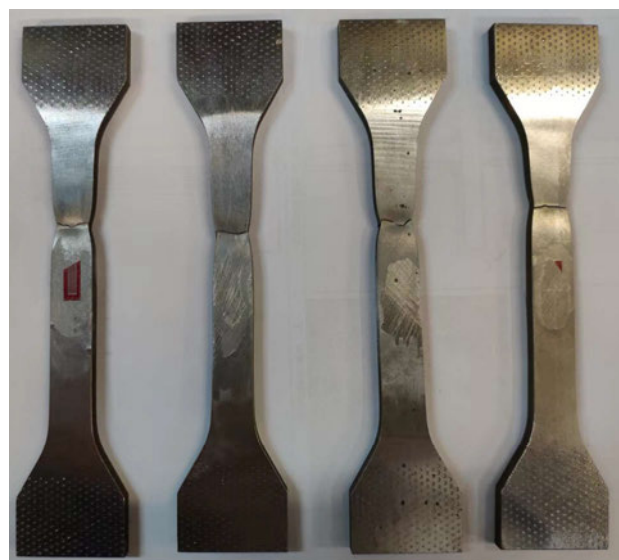
(b) Photos of fractured specimens
