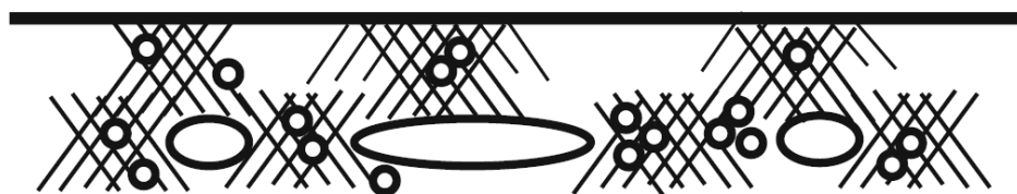
Figure 2.18 Schematic illustrations of the HESIV mechanism for the creation and clustering of vacancies forming microcracks in the strain-concentrated area close to a barrier for slip extension [47].
