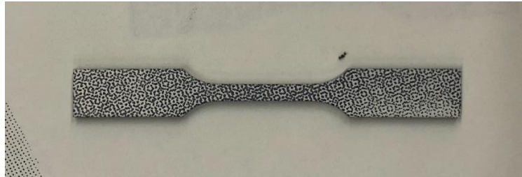
Figure 2.9 Sample surface after applying speckle pattern
