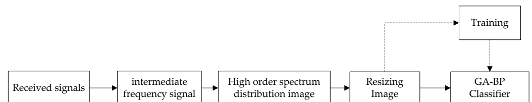
Figure 1. The structure diagram of the recognition system.
