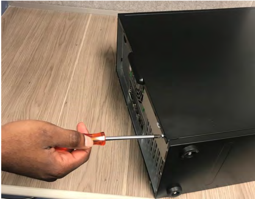
FIGURE 6.3: Unscrewing the server.
