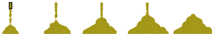
Fig. 9. Heap formation simulation at t = 1, 2, 3, 4 and 5 s from left to right. The particle insertion region is indicated with a solid line. The particle insertion is stopped at t = 4 s.
