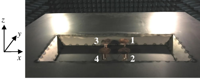
Fig. 10. Prototype of proposed quad-element MIMO antenna in Satimo SG-64.
