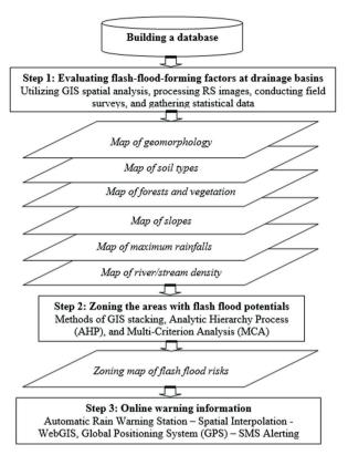
Fig. 2. Model of applying geospatial technologies in flash flood warnings in mountainous regions of Northern Vietnam
