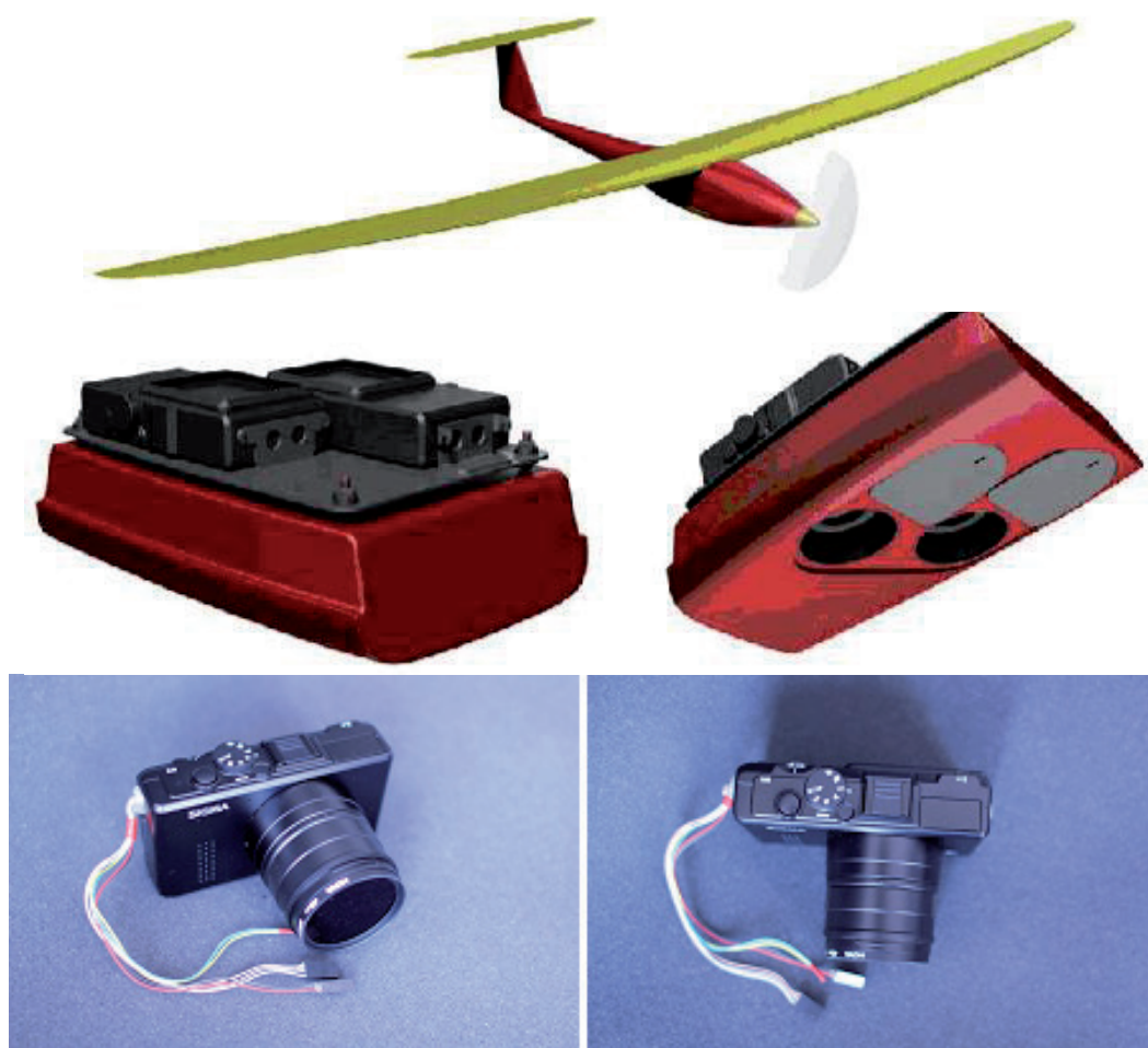
Figure 1. Unmanned aerial vehicle AVI-1, the installation of two Sigma DP2 cameras – visible wires are used to connect the controller (Source: Taxus 2010, Zmarz 2011)
