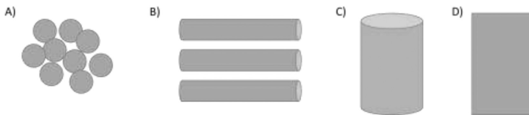
Fig. 34. Different geometries for EPCMs (a) spherical (b) tubular (c) cylindrical and (d) rectangular [153].
