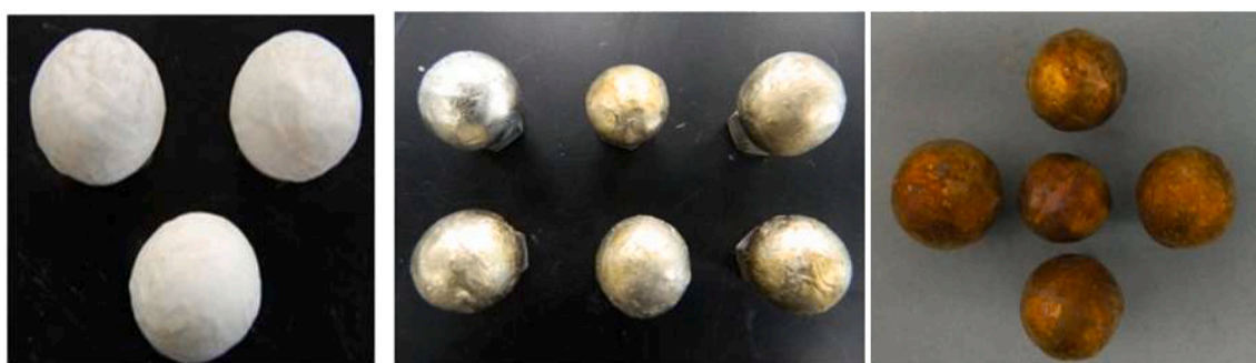
Fig. 9. Polymer encapsulated NaNO 3 (left), metal coated on polymer-NaNO 3 capsules at 356 °C after 50 cycles (middle), metal coated on polymer-NaNO 3 capsules at 356 °C after 2200 cycles (right) [59].
