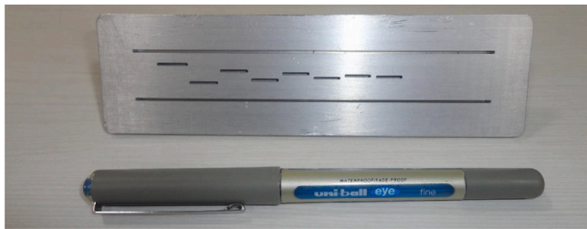
Fig. 19. Fabricated SWA antenna.
