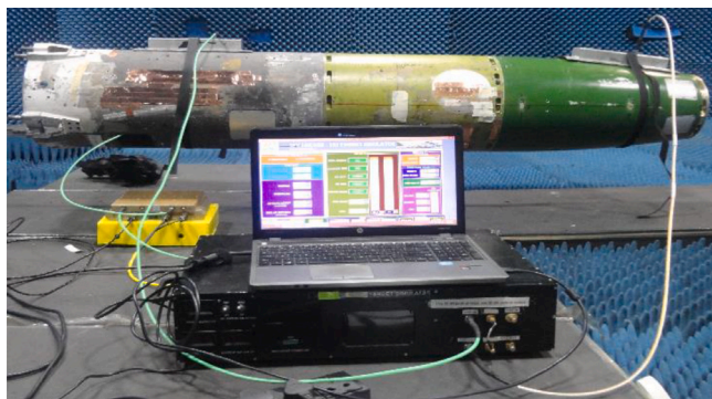
Fig. 23. Test Setup for SWA antenna.
