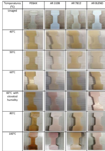
Figure 1. Pictures of unaged and aged samples of PEBAX, AR 3108 (Aritel VT3108), AR 7812 (Aritel VT7812) and 50/50 (wt./wt. %) blend of Aritel grades at various temperatures.
