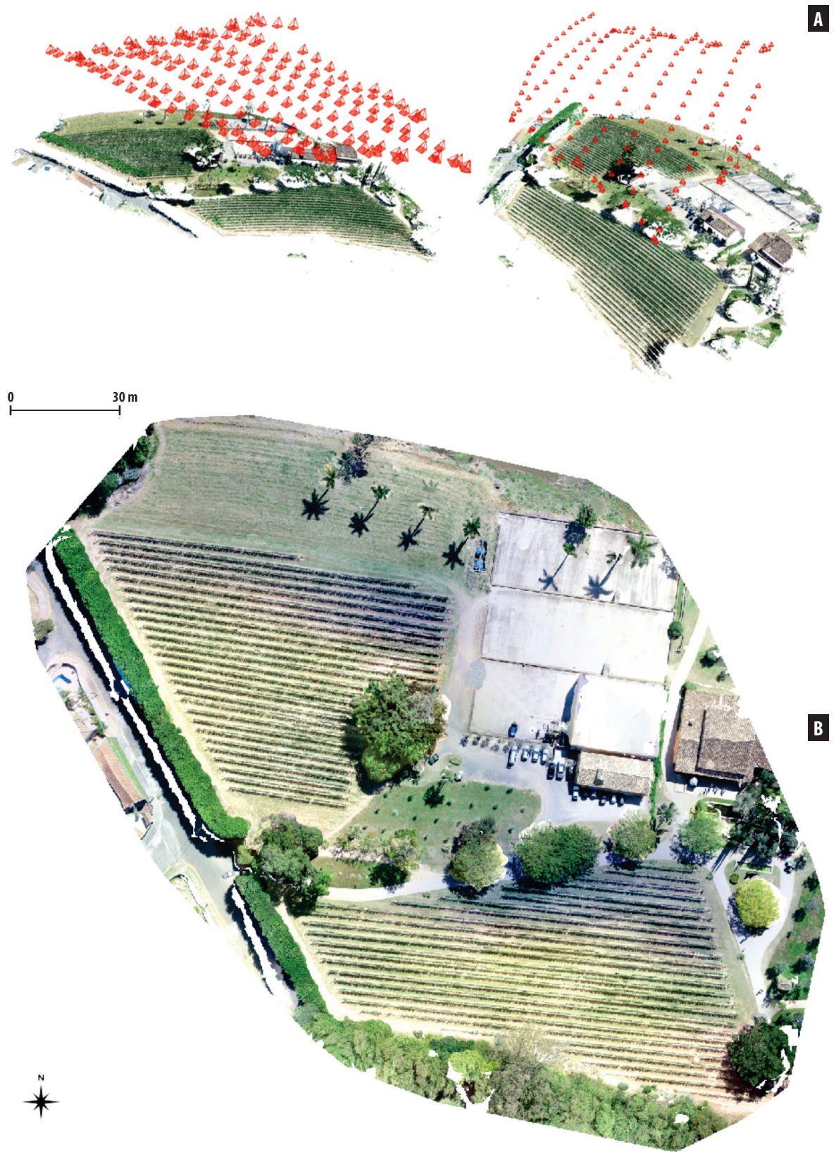
Figure 2. UAV mapping: images are used to identify the three-dimensional structure of the area, and the position and orientation of the aircraft, displayed in red (A); the geolocated three-dimensional model is then projected onto a plane, forming a map. (B).
