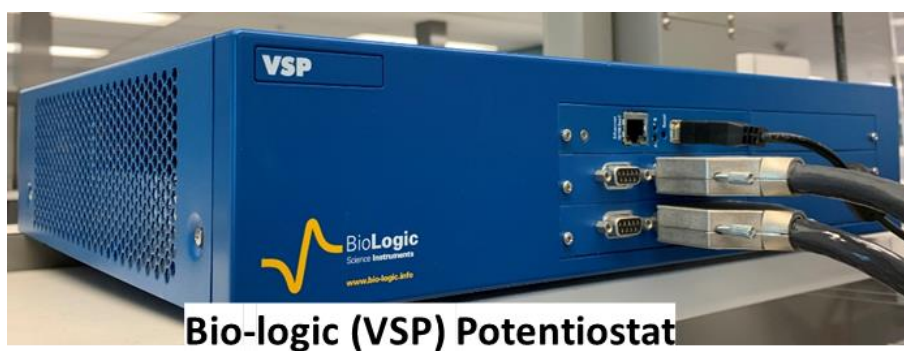
Figure 2.11 The photograph of Bio-logic VSP potentiostat.
