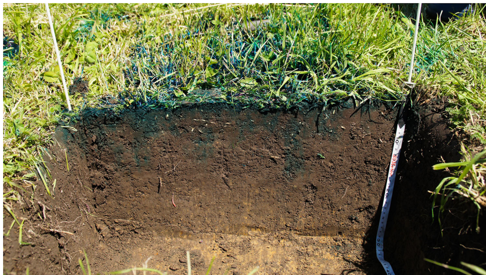
FIGURE 4 Photo of a cross section of a typical soil depth profile (depth = 30 cm) showing penetration of “brilliant blue” dye in wet soil
