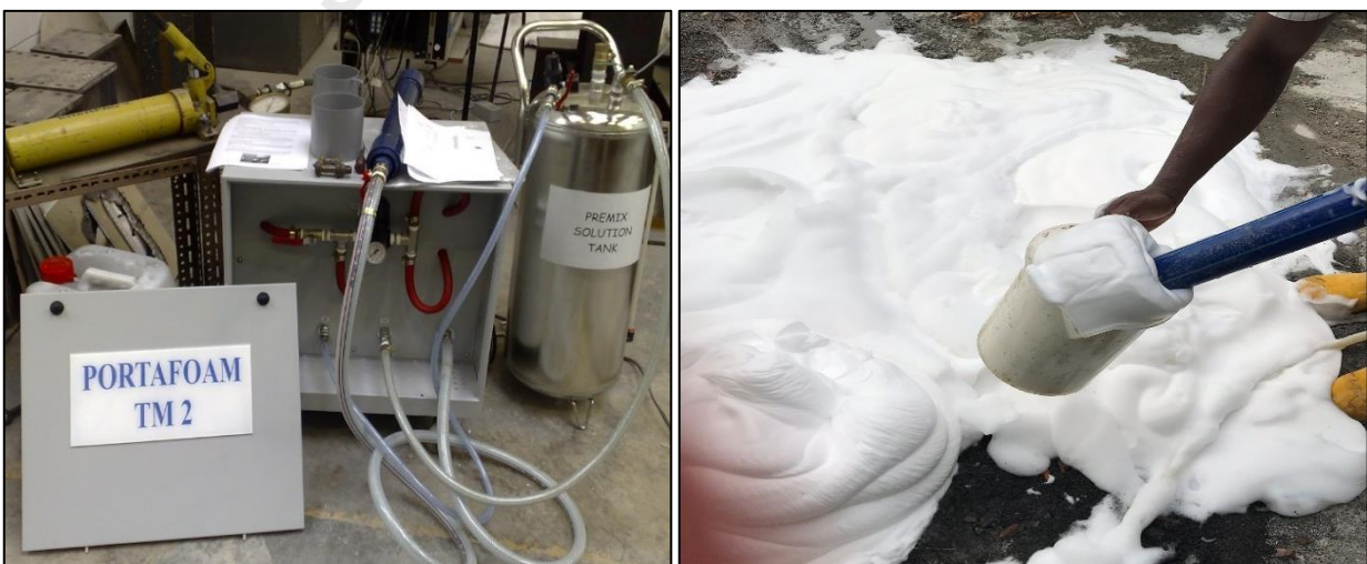
Figure 2. A Portafoam TM-2 machine was utilized to produce the stable foam
