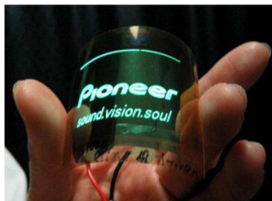
Figure 23. Flexible display on CNF substrate [259]. (Reprinted with permission from Ref. [259], Copyright 2016, copyright Tech Science Press).
