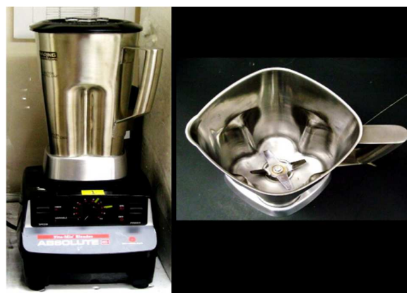
Figure 9. High-speed blender. The stainless steel bottle has a 4-blade propeller and an undulated inside wall [82]. (Reprinted with permission from Ref. [82], Copyright 2011, copyright ACS Publications).
