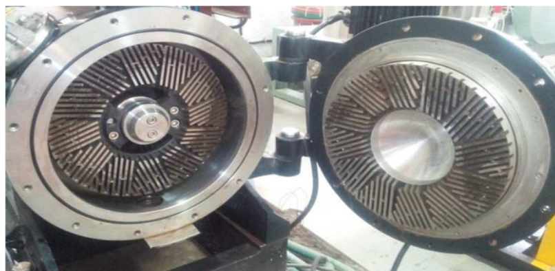
Figure 8. Disc refiner opened to show the refining surfaces [81]. (Reprinted with permission from Ref. [81], Copyright 2017, copyright Krishi).
