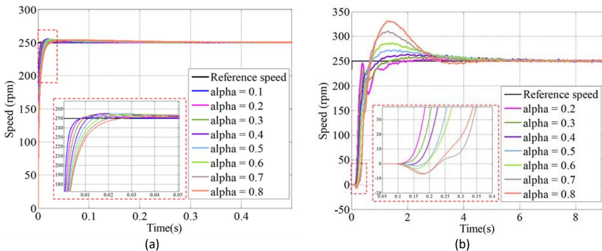
**Fig. 5.** Speed response comparison of FOSMC with various order of fractional order integration,  $\alpha$  at no load (a) simulation (b) experiment
