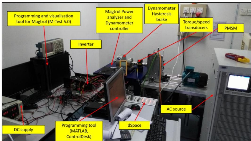
**Fig. 2.** Closed loop PMSM drive prototype
