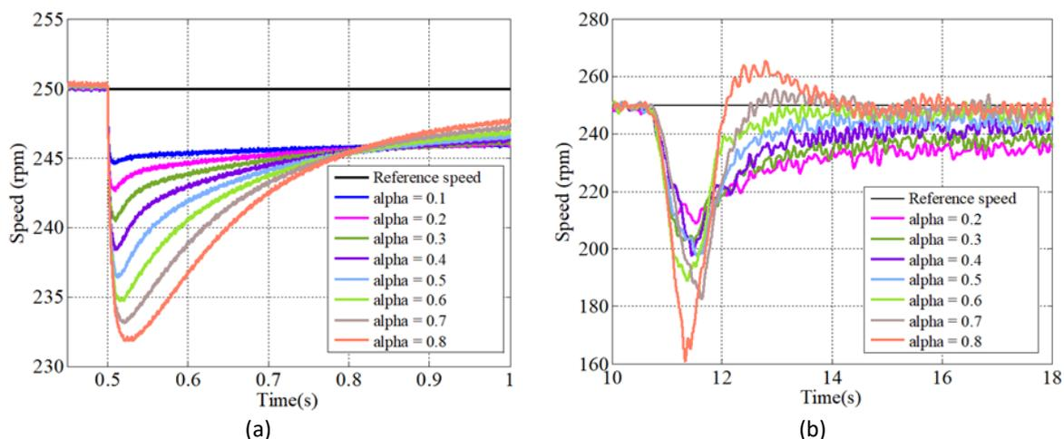
**Fig. 6.** Speed response comparison of FOSMC with various order of fractional order integration,  $\alpha$  with applied load of 0.5 Nm (a) simulation (b) experiment
