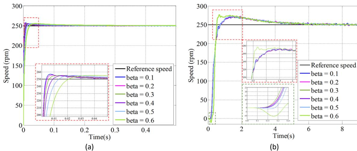
**Fig. 3.** Speed response comparison of FOSMC with various order of fractional order differentiation,  $\beta$  at no load (a) simulation (b) experiment
