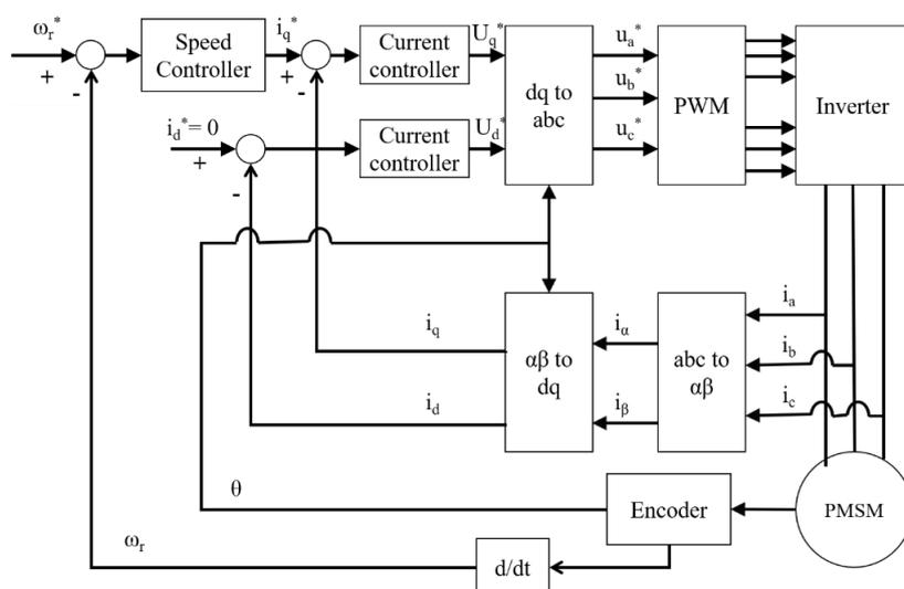
Fig. 1. Block diagram of indirect field-oriented control of PMSM
