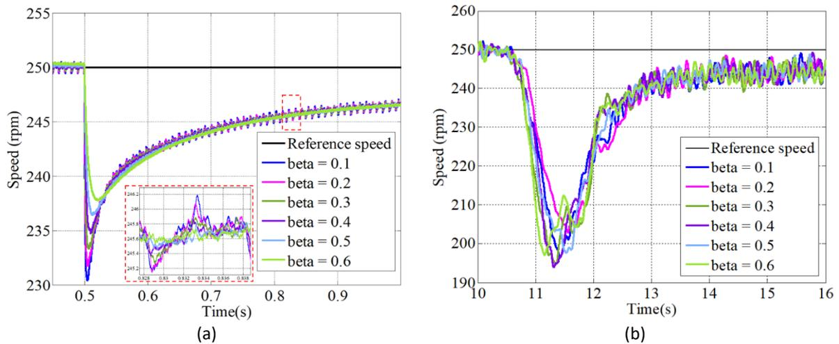
**Fig. 4.** Speed response comparison of FOSMC with various order of fractional order differentiation,  $\beta$  with applied load of 0.5 Nm (a) simulation (b) experiment
