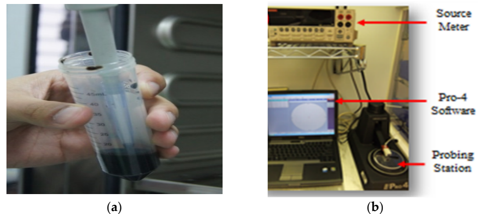
Figure 5. (a) Liquid reduced graphene oxide (b) Four-point probe device.
