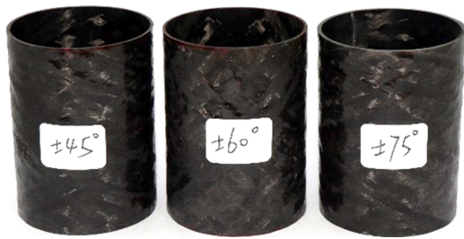
Fig. 3. Thin-walled filament wound CFRP tubes fabricated by laboratory scale 3-axis winding machine.
