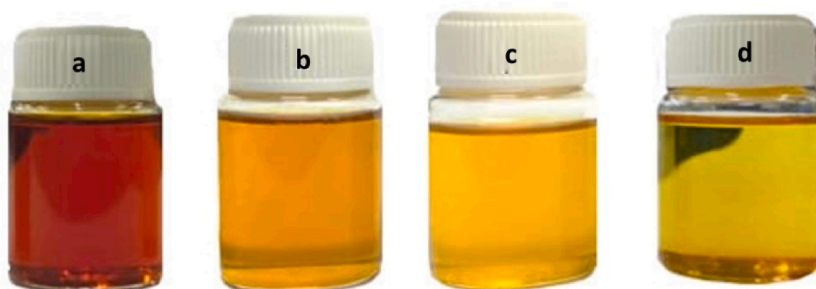
Fig. 5. Liquid products from (a) PP pyrolysis and reforming process using Ni/ZAA with Ni loadings of 5.0 wt% (b), 15% wt.% (c), and 20 wt% (d).
