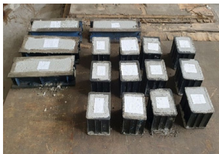
(c) Each concrete cube and concrete beams were marked
