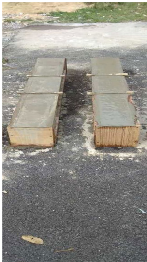
Fig. 8 Casted reinforced concrete beam
