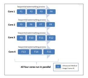
Figure 2. Multi-frame watermarking scheme
