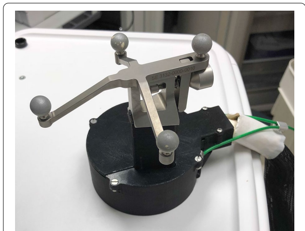
Fig. 1 Handheld SiPM gamma camera with four reflecting spheres
