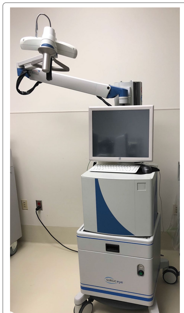
Fig. 2 The investigational camera declipse®SPECT system. The SiPM camera is mounted in a holder behind the monitor when not in use
