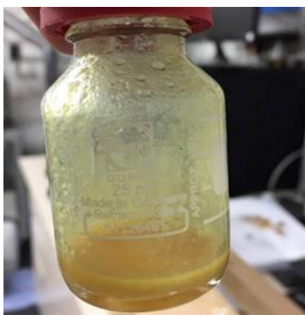
Figure 3.12 - Oil extracted by supercritical CO 2 at 30 MPa and 60 °C.
