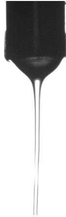
Figure 5.4 - Pendant drop of model oil in a CO 2 atmosphere at 25 MPa.
