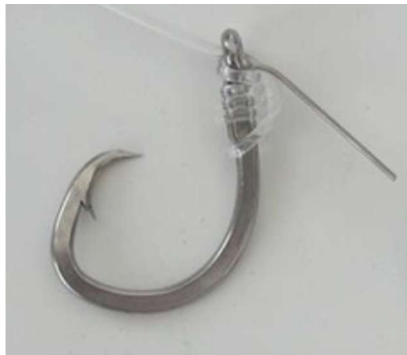
Figure 4. Circle hook modified with a wire appendage.
