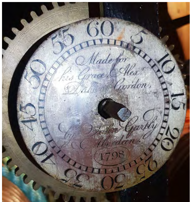
Figure 5.11. Hand-setting dial inscribed 'Made for his Grace, Alexr. Duke of Gordon by John Gartly Aberdeen 1798', interior of clock tower, Bellie Kirk, Fochabers. Author's photograph.
