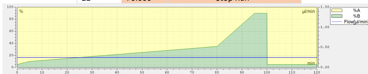
FIGURE 9 – METHOD OF CHROMATOGRAPHIC SEPARATION FOR TMT10PLEX
