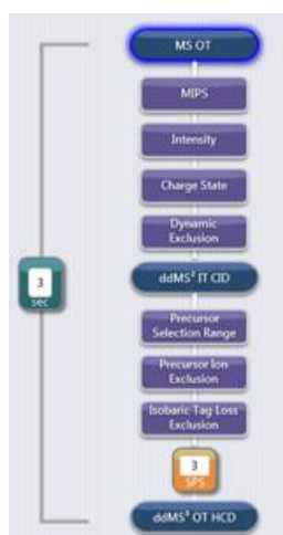
FIGURE 10 – SYNCHRONOUS PRECURSOR SELECTION MS3 METHOD
