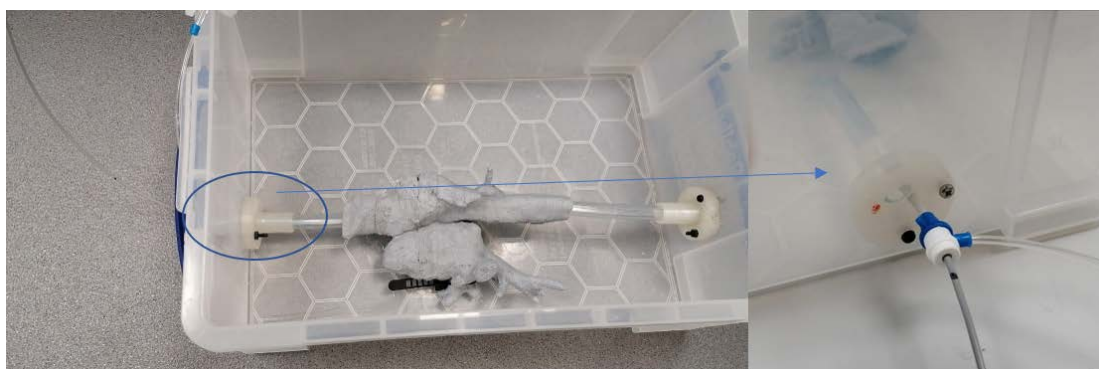
Figure 5.3. Initial design of atrial ablation simulator
