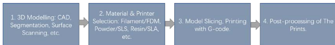
Figure 1.1 General principles of 3D printing
