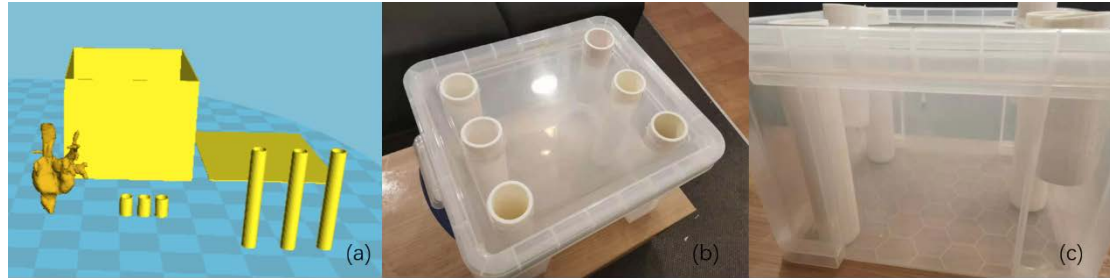
Figure 5.5. Upgraded assembly of atrium model container with patch holders
