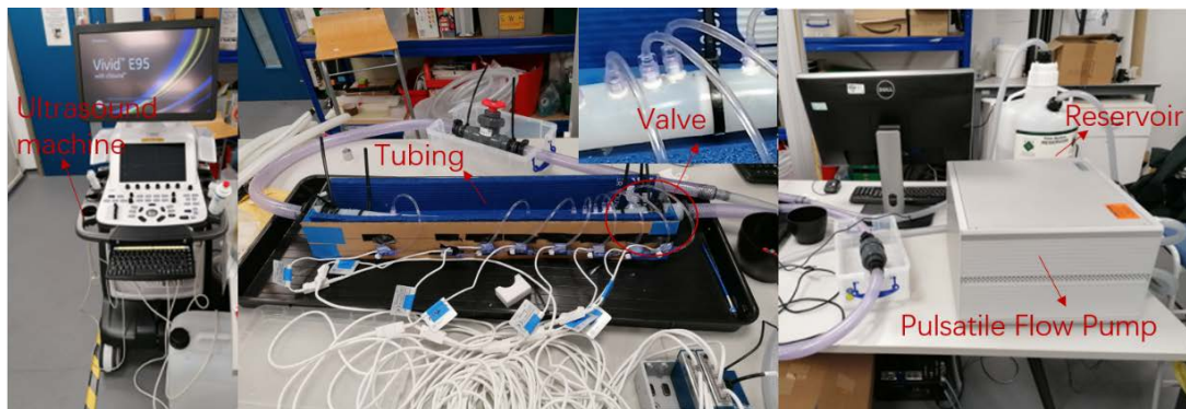
Figure 6.16: Ultrasound imaging platform for valve experiments with a pulsatile flow pump
