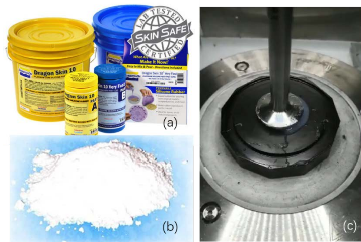
Figure 3.15: Experimental setup for silicone materials' rheological characterisation: (a) two-part Dragonskin 10 RTV silicone (Bentley Advanced Materials, UK); (b) used hydrophobic fumed silica powder; (c) Anton-Paar MCR92 rheometer, test in progress
