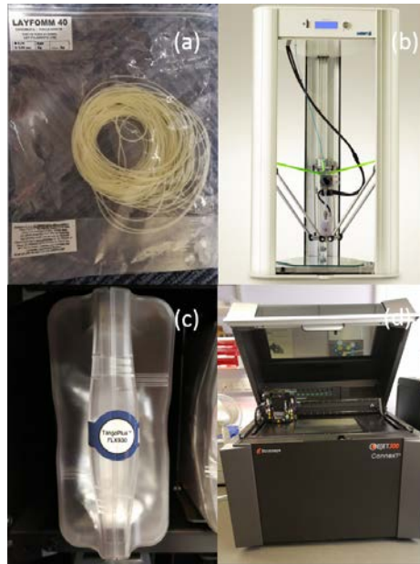
Figure 4.4. 3D Printing: Layfomm40 (a) used by the WASP Delta 2040 printer (b) and Tango Plus (c) printed on a PolyJet Objet500 printer (d)
