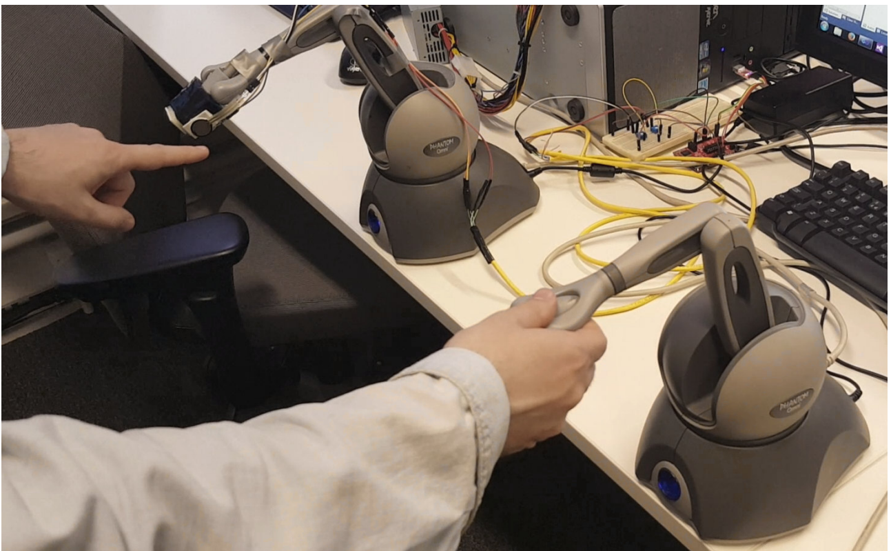
Figure 3.2: Two Phantom Omni devices (as master and slave) operating in position-force configuration over a network using an SDN-capable switch.
