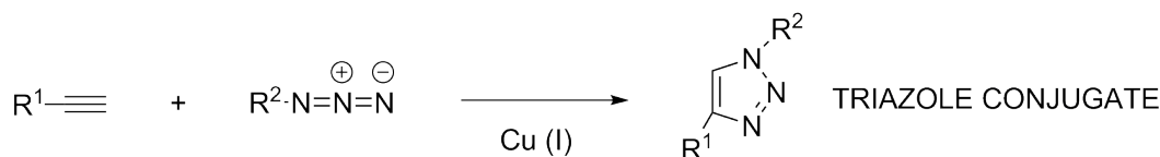
Scheme 5.1: Copper catalysed alkyne azide cycloaddition
