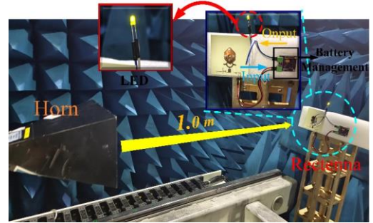
Fig. 16. The ambient electromagnetic energy is supplied by a source at the left end, and at the right end an all polarization rectenna connected to a battery management module. The battery management module stabilizes the voltage value and light up the light emitting diode.
